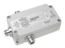
An antenna splitter may be used to drive multiple GPS receivers using a single antenna. With built-in amplification to overcome splitter losses, the Active Splitters may be conveniently cascaded without adding separate amplifiers and bias-tees between splitters. Power is conveniently obtained from the GPS receiver(s) connected to the amplifier, eliminating the need for a separate dc power supply and wiring.
