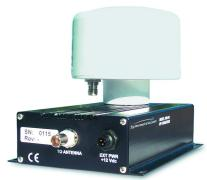
Use the GPS Down/Up converter for cable runs of 250 to 1500 feet (75 m to 457 m). GPS signal down/up conversion is required when signal losses in the antenna cable limit the distance between the receiver and the antenna assembly. The Down/Up Converter may also work with non-Symmetricom L1 GPS receivers. The signal output from the converter is L1 C/A code that can be decoded by any L1 GPS receiver.
